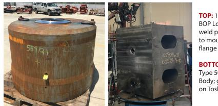
**TOP:** 18-5M Type 52 BOP Lower Housing; weld prep completed to mount weld neck
